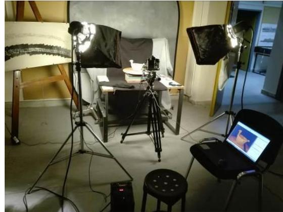
Figure 3: Focus stacking acquisition set-up
