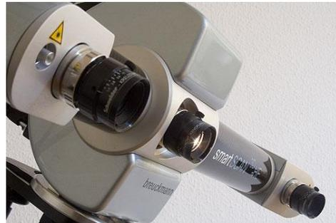
Figure 1: SmartSCAN 3D-HE structured light system (Breuckmann, 2017)
