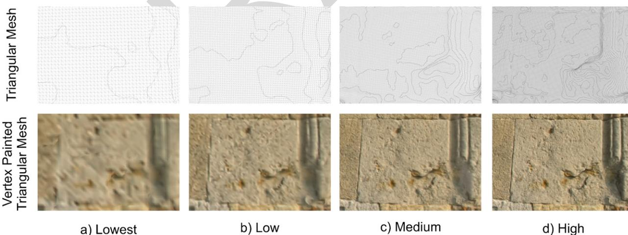
Fig. 1. Different LODs of the triangular mesh.
