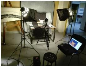
Figure 3: Focus stacking acquisition set-up
